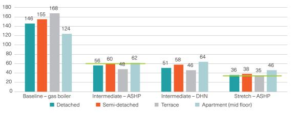
Key Green line indicates the target: Intermediate = 60; Stretch = 35 kWh/m<sup>2</sup>/year ASHP = air source heat pump
