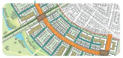
Extending the swale network to include primary and secondary streets reduces embodied carbon from the stormwater network, whilst also increasing the provision of 'blue/green networks'. This highlights the general principle of reducing materials used, in place of naturebased solutions that help deliver holistic benefits, including climate resilience.
