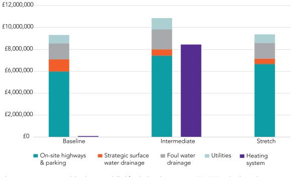
Please note, a gas network has been modelled for the baseline scenario (£95,000) and a district heat network option for the intermediate scenario (£8.5mil), separate to the masterplan costs. This is the heat infrastructure associated with the masterplan. All heating systems within the curtilage of homes is covered in the homes' analysis, including the on-plot air source heat pumps in the stretch scenario.
