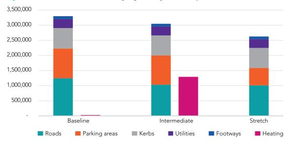
Figure 8: Total embodied carbon results (kgCO<sub>2</sub>e; heating has been separated)
