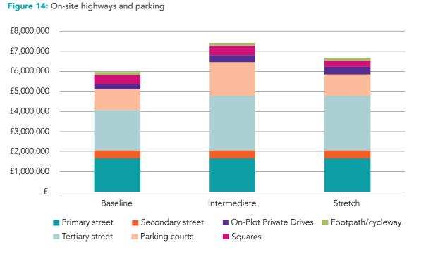
Overall, the cost uplift between the baseline and stretch scenarios for highways and parking is moderate at 12% (from £6m to £6.7m).
