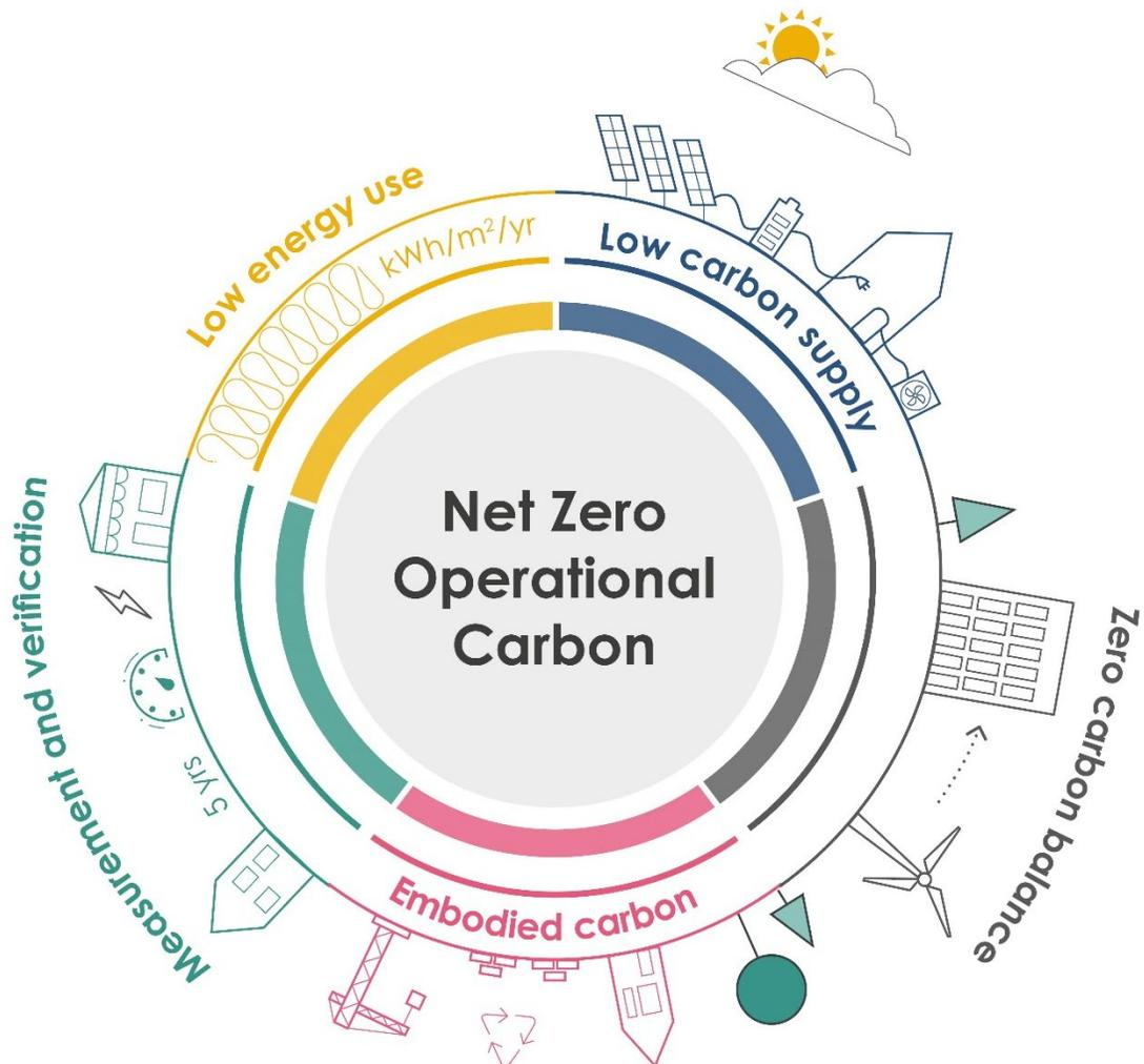
**Figure 1:** The component elements of achieving a net zero carbon new home (Credit: LETI)
